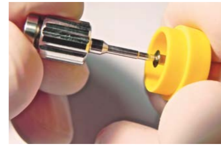
1. Closure screw anchoring the implant to the cap. Removed with the aid of a screwdriver for K - KT - KE - TTI - TTx hexagonal screwdriver. Use the TORX screwdriver for TTc implant.
