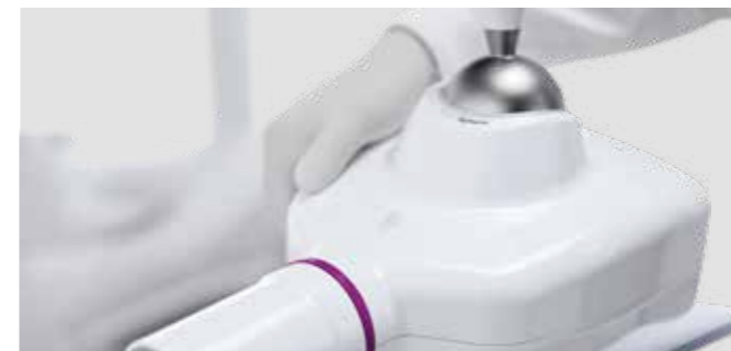
RXDC - HyperSphere technology Incorporated on the dental unit, the X-ray unit and handheld control unit require no additional installation points. Thanks to a combination of 30 cm collimation and a 0.4 mm focal spot, parallelism is excellent and images are pin sharp. Locked and unlocked by touch-sensitive pads, the tube head rotates freely around the spherical joint.
